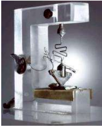
The first transistor(1948)
