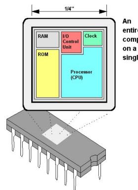
An entire computer on a single chip. • Intel, *founded* in 1968 by Robert Noyce and Gordon Moore, introduces a "Computer on a chip," the 4004 four-bit microprocessor, design by Frederico Faggin, Ted Hoff, and Stan Mazor. It can execute 60,000 operations per second and changes the face of modern electronics by making it possible to include data processing hundreds of devices. A 4004 provides the computing power for NASA's Pioneer 10 *spacecraft*, launched the following year to survey *Jupiter*.
